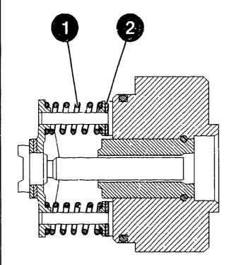
The parts set (plunger return spring) is being added to the service-parts list under item 50/804.
